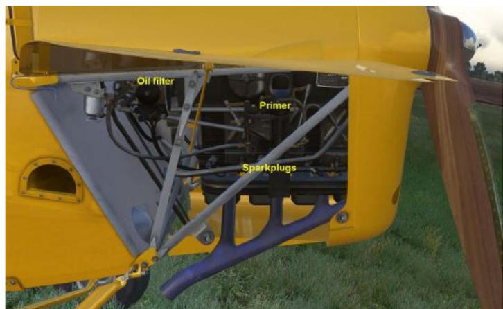
The Tiger Moth uses an AUTO-KLEAN oil filter. Rotate the lever on the oil filter once every day.
